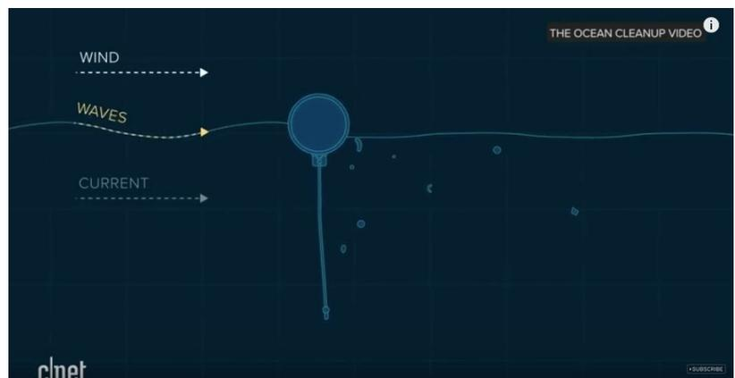
Crowdfunded at that time by 38000 people from many countries, the aim was to produce a passive system that gathers large amounts of waste from the ocean. The theory is as impressive as it is simple. Guided by natural currents a large concave boom over 600 metres long and three metres in depth moves more quickly than the materials floating on or near the surface, thus gathering those items in its path.
